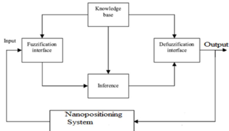
Figure 6 Block Diagram of Fuzzy Logic Based Nanopositioning System
