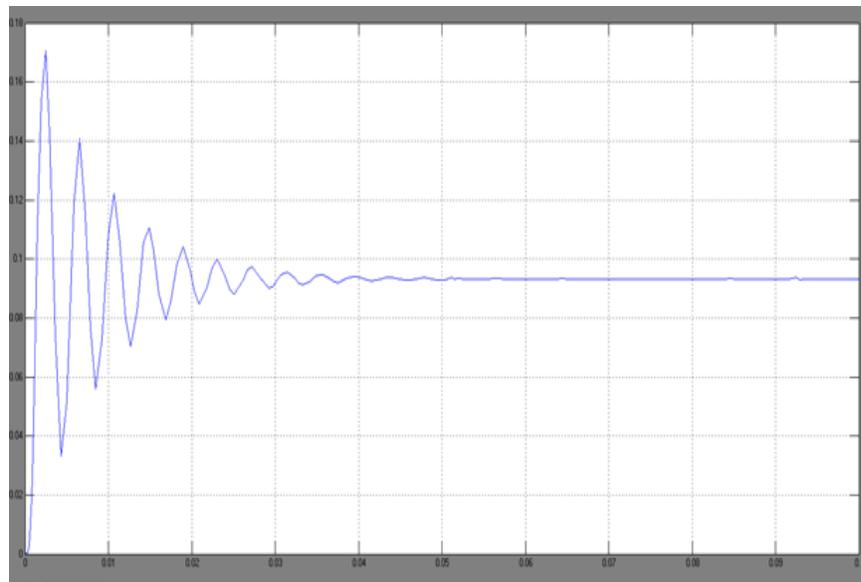
Figure 11 Time Response of Nanopositioning System Using Fuzzy Based PID Controller
