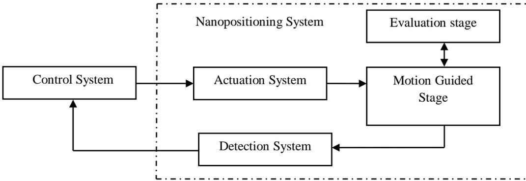
Figure 1 Nanopositioning System
