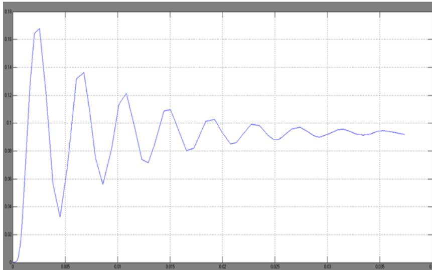
Figure 10 Time Response of Nanopositioning System Using Fuzzy and PI Controller
