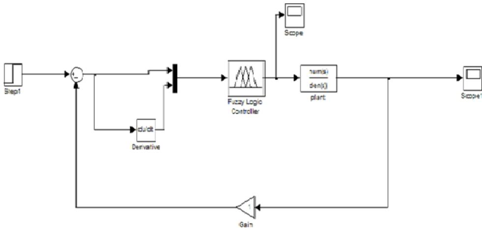
Figure 7 Simulink Model of Nanopositioning System Using Fuzzy Logic Controller
