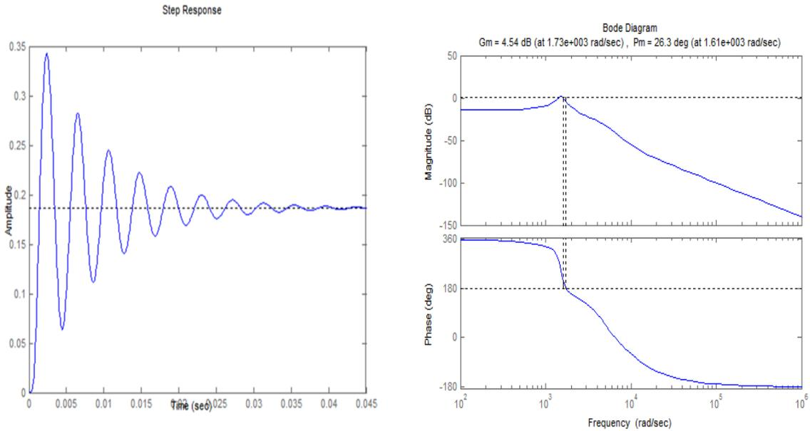
Figure 2 Time and Frequency Response of Open Loop Nanopositioning System
