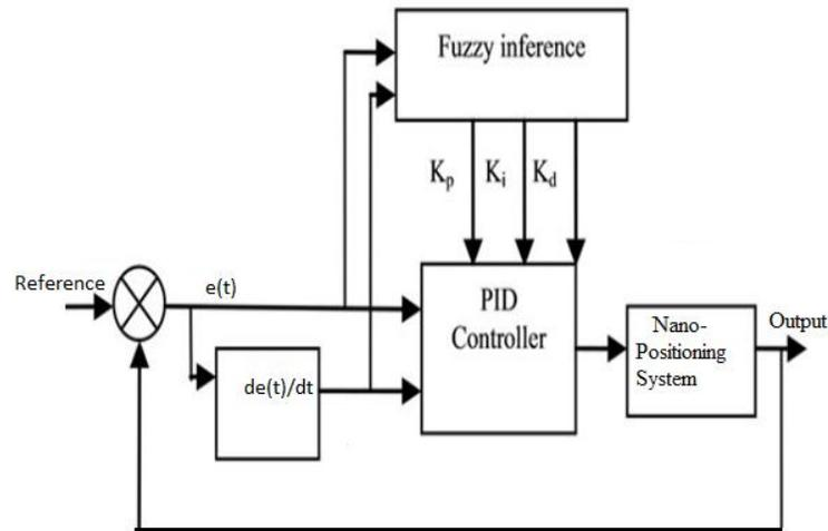
Figure 5. Configuration of Fuzzy PID Controller
