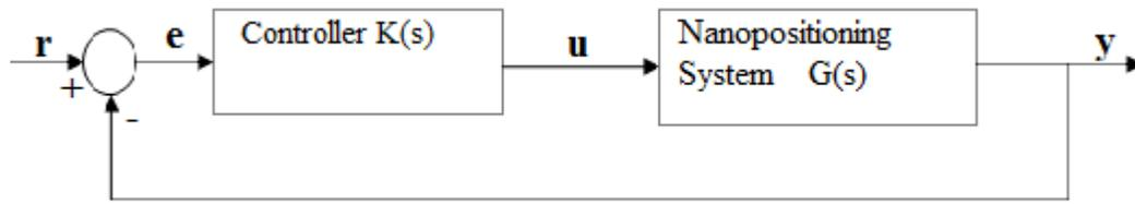
Figure 3 Closed Loop Nanopositioning System
