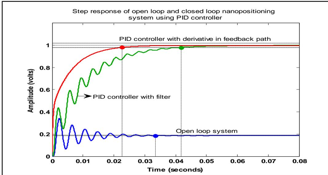
Figure 4 Closed Loop Time Response Using PID Controller Based on Z-N Tuning
