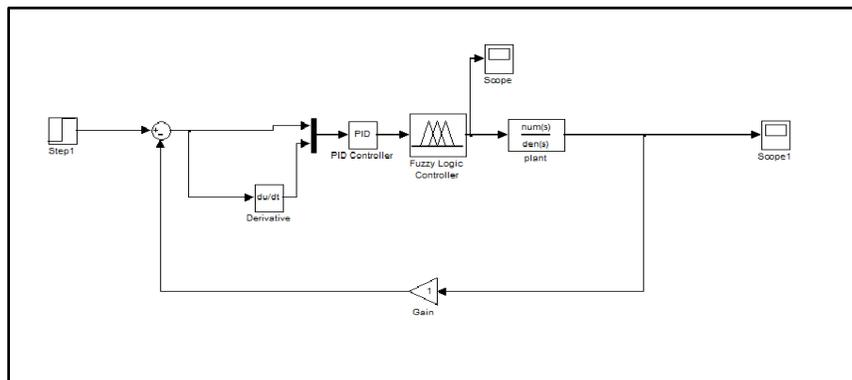
Figure 9 Simulink Model of Nanopositioning System Using Fuzzy Based PID Controller
